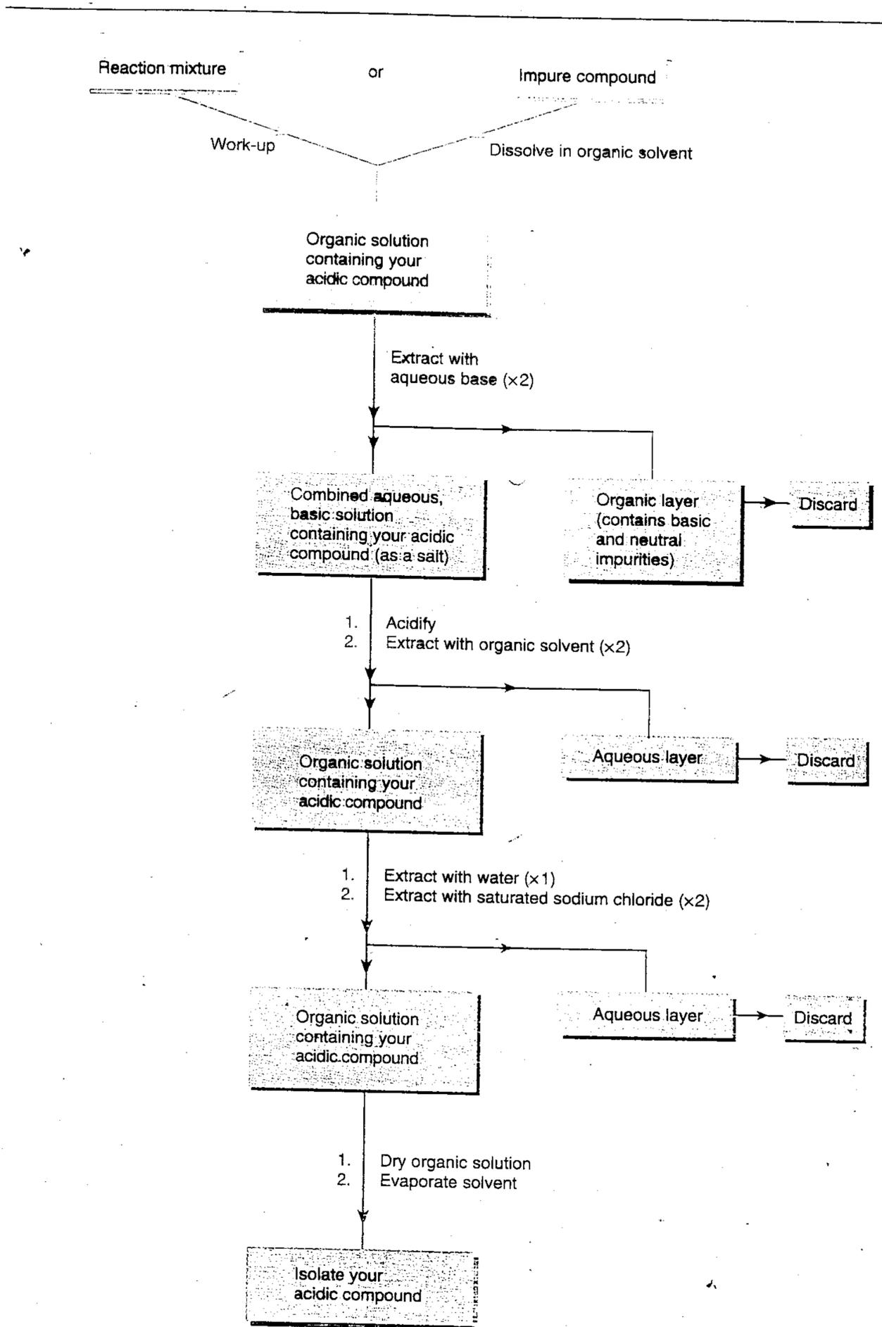
**Fig. 3.38** Extraction protocol for the isolation and purification of an acidic organic compound.
