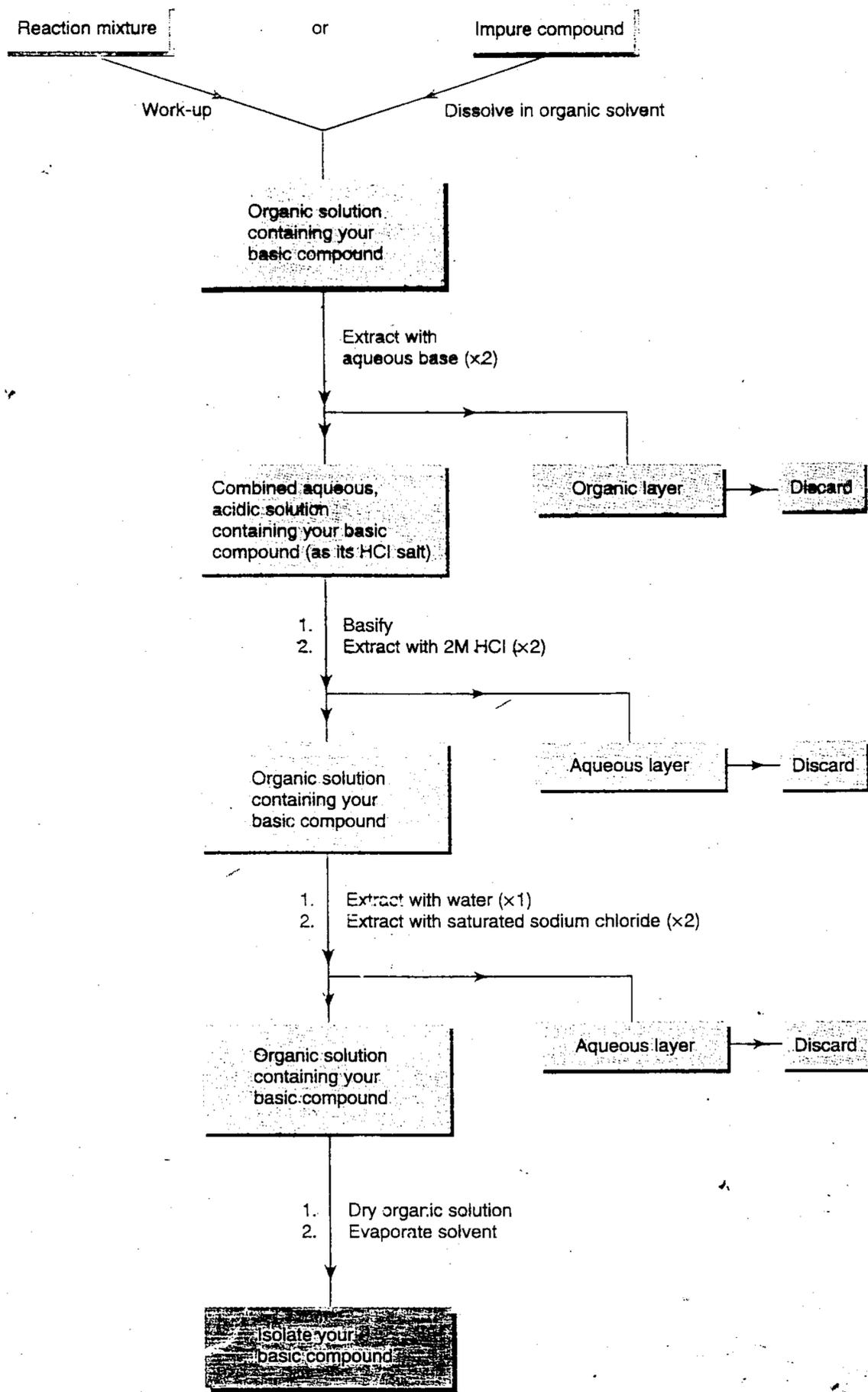
**Fig. 3.39** Extraction protocol for the isolation and purification of a basic organic compound.
